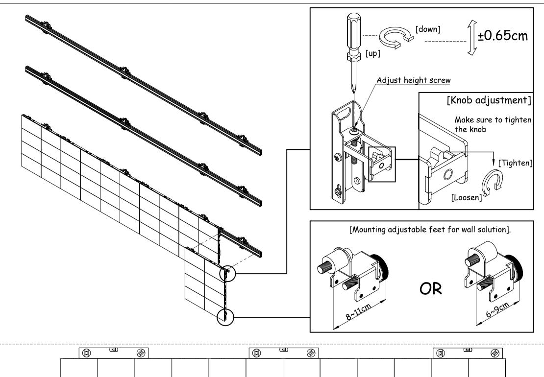
After splicing, adjust the dvLED displays to the same level.
